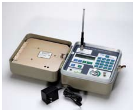
Avtech's battery powered CTS-700 Ramp Tester contains a built in transmitter and uses VHF or HF signals, transmitted directly to the aircraft, to conveniently test the SELCAL system at the aircraft without any intervention from the tower or ARINC
